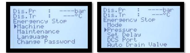
You may now adjust the load and unload values to the desired settings for your application by hitting enter and using the up/down arrows
