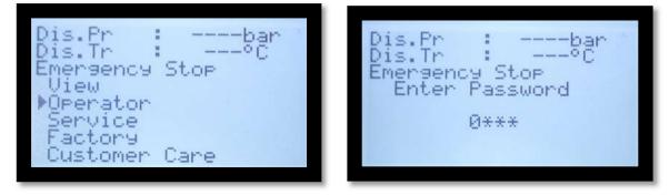
Once in the **OPERATOR** menu, select **MACHINE** by pressing enter, then select **PRESSURE** by pressing enter.
